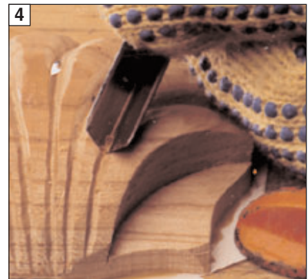
4 Carve the lobe lines with a V-tool, then round over the sides of the lobes to separate them. The wings have been cut to about \frac{1}{4} " thick.
